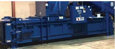
Installation would include the hiring of a construction firm to lift the baler off the shipping flat, move it to its designated place of operation, anchoring it into the concrete, installing any attachments that were removed for shipping, connecting all electrical equipment (disconnect and conduit), and installing hydraulic oil if it was removed for shipping. If a new unit is purchased, final electrical connections and training from the sales staff comes with the purchase.
