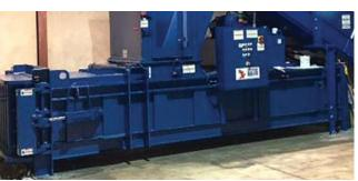
Installation would include the hiring of a construction firm to lift the baler off the shipping flat, move it to its designated place of operation, anchoring it into the concrete, installing any
